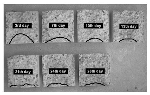
FIGURE 4. The seepage shape in various time periods after the creation of specimens.
