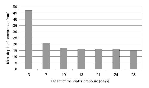
FIGURE 5. Relation between seepage and loading time.
