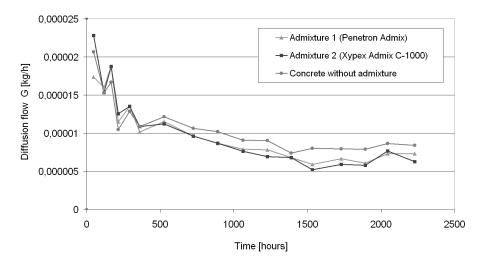
FIGURE 8. Diffusion flow of water vapor through the specimens during the test.
