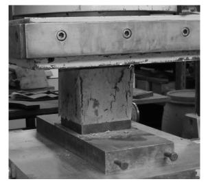
FIGURE 9. Loading of test specimen in a hydraulic press.
