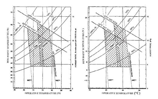
Fig. 10: Acceptable ranges of operative temperature and humidity for people in typical summer and winter clothing during light, primarily sedentary activity (≤ 1.2 met) according to ANSI/ASHRAE Standard 55-1992. The operative temperature ranges are based on a 10 % dissatisfaction criterion.
