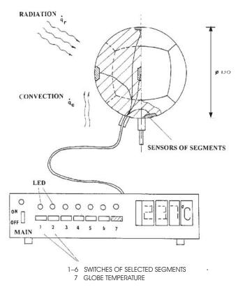
Fig. 18: Stereothermometer
