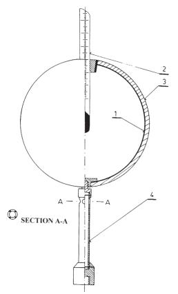
Fig. 8: The Vernon-Jokl globe thermometer (1 thin copper globe, 2 thermometer, 3 polyurethane, 4 fastening stand)
