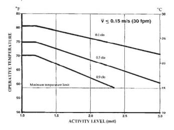
Fig. 15: Optimum operative temperatures for active people in environments with a low air speed  $v \le 0.15$  m/s (30 fpm) according to ANSI/ASHRAE Standard 55-1992
