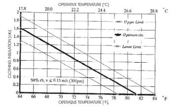
Fig. 9: The recommended range of clothing insulation providing acceptable thermal conditions at a given operative temperature for people during light, primarily sedentary activity (≤ 1.2 met) according to ANSI/ASHRAE Standard 55-1992. The limits are based on a 10 % dissatisfaction criterion.
