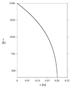
Fig. 4: Temperature profile within a foam concrete wall in a wide temperature range. Parameters: d=0.2 m,  $T_1=1500$  K,  $T_2=400$  K,  $a=6\cdot10^7$  Wm $^{-1}$ K $^{-3}$ ,  $T_0=165$  K,  $\lambda_0=0.0570$  Wm $^{-1}$ K $^{-1}$ .
