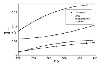
Fig. 2: Parabolic behaviour of thermal conductivity in a wider temperature range
