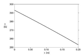
Fig. 3: Temperature profile within the foam concrete wall in a narrow temperature range. Parameters:  $d=0.2\,$  m,  $T_1=293\,$  K,  $T_2=253\,$  K,
