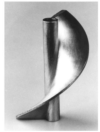
Fig. 3: Screw agitator used in experiments
