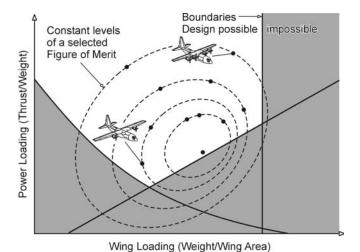
Fig. 4: Design diagram with plottings of evaluable solutions
