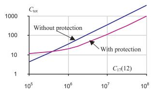
Fig. 2: Expected total cost  $C_{tot}$  versus cost  $C_{17}(12)$  due to structural collapse for  $p_{fi.\,5} = P(H_2) = 0.01$
