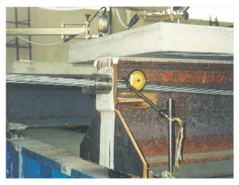
Fig. 4: Structural detail at the end support section showing the head of the anchorage device acting against a rigid steel plate
