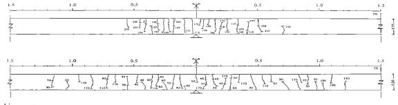
Fig. 10: Cracking pattern
