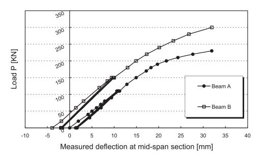
Fig. 8: Load-deflection response for Beam B (prestressed) & beam A (non-prestressed)
