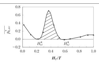
Fig. 6: Axial profile of the dimensionless peripheral component of dynamic pressure affecting a radial baffle along its height (h/T = 0.33)
