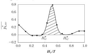
Fig. 7: Axial profile of the dimensionless peripheral component of dynamic pressure affecting a radial baffle along its height (h/T = 0.48)
