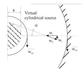
Fig. 5: Turbine impeller as a cylindrical tangential jet
