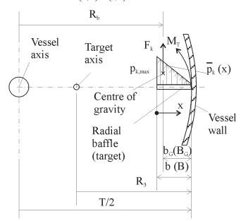
Fig. 8: Radial profile of baffle loading
