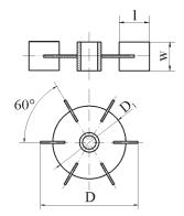
Fig. 2: Standard Rushton turbine disk impeller  $(D/T = 1/3, w/D = 0.2, D_1/D = 0.75, l/D = 0.25)$
