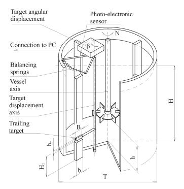
Fig. 1: Sketch of a flat-bottomed agitated pilot plant mixing vessel with four radial baffles at the wall and axially located standard Rushton turbine impeller and sketch of measurement of local peripheral force affecting the trailing target (H/T = 1, h/T = 0.33, 0.48, b/T = 0.1,  $h_T = 10$  mm, B = 28 mm)
