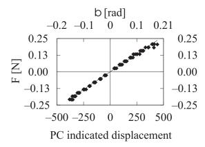
Fig. 3: Results of mechanical calibration of balancing springs
