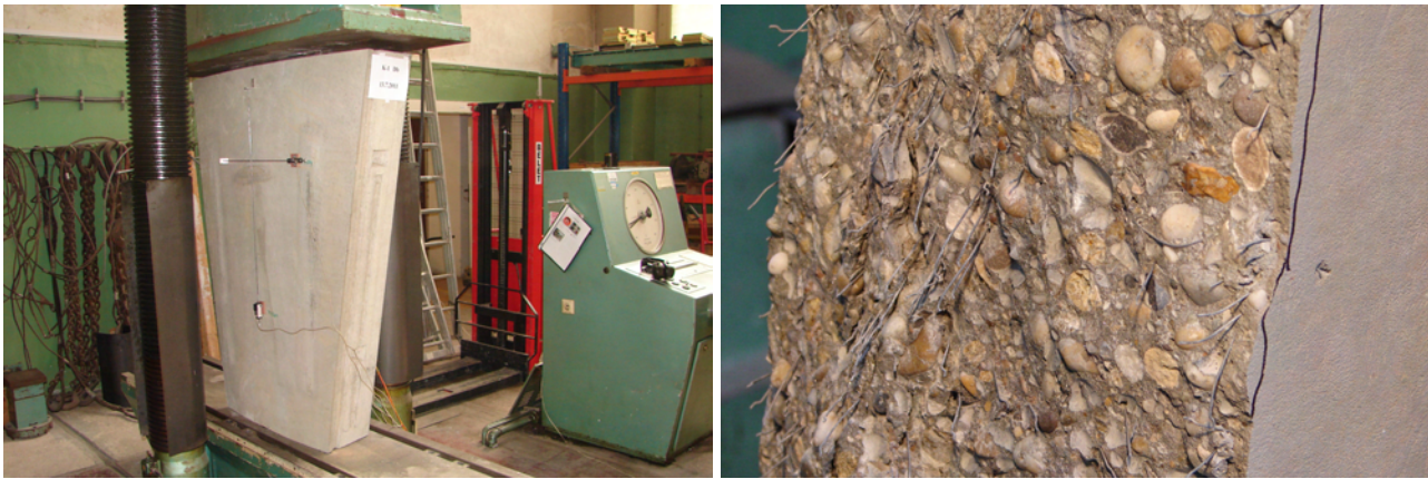
FIGURE 6. Key segment compression (left: segment installed in the test machine; right: detail of the fractured surface).
