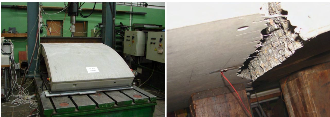
FIGURE 7. Segment bending (left: segment installed in the test machine; right: a detail of the fractured surface).
