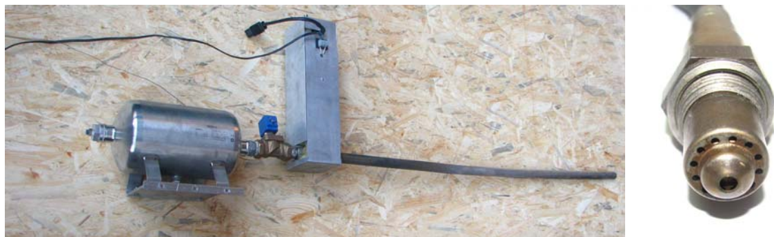
Figure 1: The extraction line and the head of the \lambda -sensor
