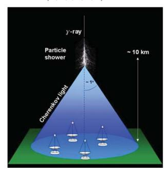
Fig. 2: Illustration of the air shower technique  $http://icc.ub.edu/gp\_oa.php$
