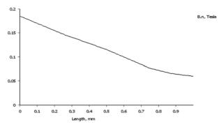
Fig. 34: Normal flux density diagram in the stator core area, through the magnet axis
