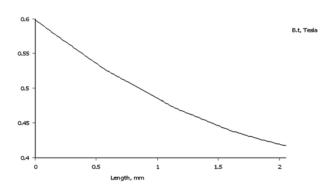
Fig. 31: Tangential flux density diagram in the winding area, through the magnet axis
