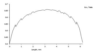
Fig. 30: Normal flux density diagram in the air-gap area, on polar pitch
