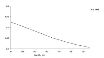
Fig. 16: Tangential flux density diagram in the air-gap area, through the magnet axis
