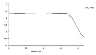
Fig. 24: Normal flux density diagram in the rotor hub, in the neutral area  $\,$
