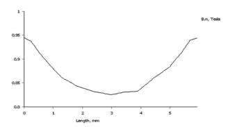
Fig. 14: Normal flux density diagram, transversal on the magnet, in the base of the middle area
