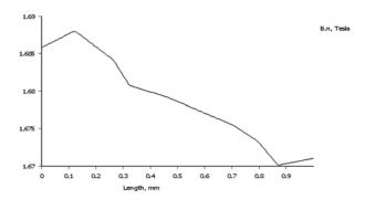
Fig. 35: Normal flux density diagram in the stator core area
