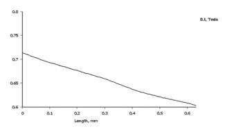
Fig. 29: Tangential flux density diagram in the air-gap area, through the magnet axis
