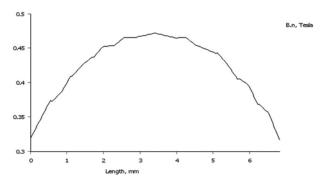
Fig. 19: Normal flux density diagram in the winding area, on polar pitch
