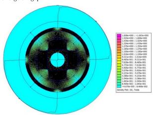
Fig. 6: Magnetic field distribution
