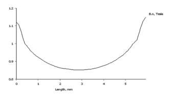
Fig. 26: Normal flux density diagram, transversal on the magnet, in the base of the magnet area
