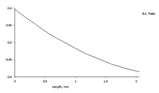
Fig. 45: Tangential flux density diagram in the winding area, through the magnet axis
