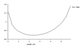
Fig. 40: Normal flux density diagram, transversal on the magnet, in the base of the magnet area
