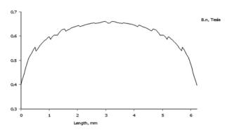
Fig. 17: Normal flux density diagram in the air-gap area, on polar pitch
