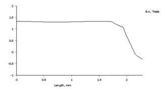
Fig. 11: Normal flux density diagram in the rotor hub, in the neutral area
