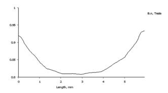
Fig. 27: Normal flux density diagram, transversal on the magnet, in the middle area
