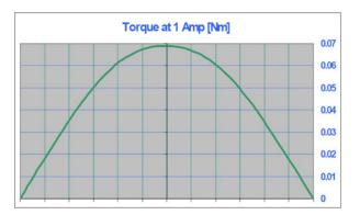
Fig. 7: Torque versus electric angle diagram  $\,$
