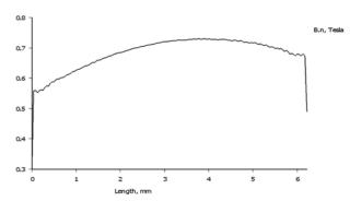
Fig. 42: Normal flux density diagram, transversal on the magnet, at the limit to the air-gap area
