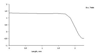
Fig. 38: Normal flux density diagram in the rotor hub, in the neutral area  $\,$
