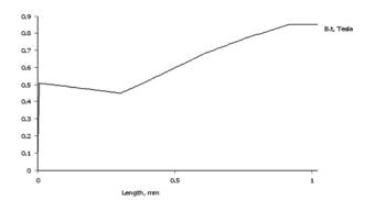
Fig. 23: Tangential flux density diagram in the rotor hub, through the magnet axis
