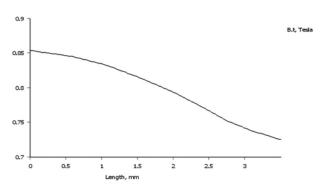
Fig. 12: Tangential flux density diagram, on the magnet, through the magnet axis
