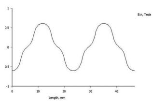
Fig. 8: Flux density diagram in the air-gap, in the proximity of the permanent magnet
