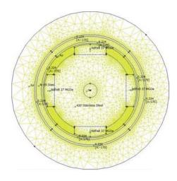
Fig. 1: An example of a limited angle torque motor with a small air-gap
