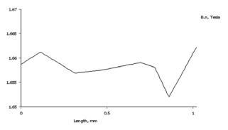
Fig. 49: Normal flux density diagram in the stator core area
