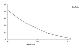
Fig. 20: Tangential flux density diagram in the stator core area, through the magnet axis
