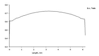
Fig. 28: Normal flux density diagram, transversal on the magnet, at the limit to the air-gap area
