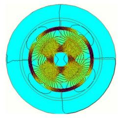
Fig. 36: Torque motor with a large air-gap in load conditions at  $5\mathrm{A}$  — distribution of the magnetic field
