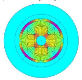
Fig. 9: Torque motor with a large air-gap in no load conditions — magnetic field distribution
