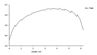
Fig. 44: Normal flux density diagram in the air-gap area, on polar pitch
