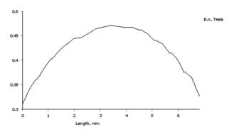
Fig. 32: Normal flux density diagram in the winding area, on polar pitch
