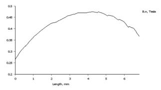
Fig. 46: Normal flux density diagram in the winding area, on polar pitch
