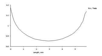
Fig. 13: Normal flux density diagram, transversal on the magnet, in the base of the magnet area  $\,$
