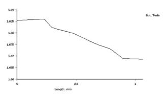
Fig. 21: Normal flux density diagram in the stator core area  $\,$
