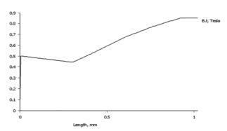
Fig. 37: Tangential flux density diagram in a rotor hub, through the magnet axis
