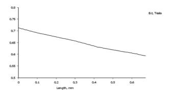
Fig. 43: Tangential flux density diagram in the air-gap area, through the magnet axis
