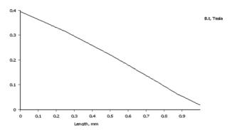
Fig. 47: Tangential flux density diagram in the stator core area, through the magnet axis
