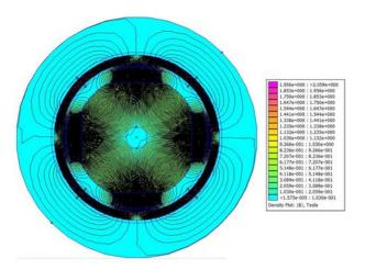
Fig. 2: Magnetic field distribution
