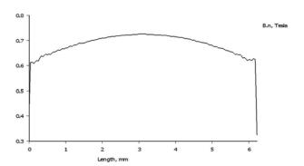
Fig. 15: Normal flux density diagram, transversal on the magnet, at the limit to the air-gap area  $\,$
