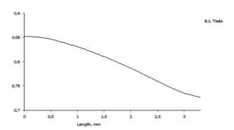
Fig. 25: Tangential flux density diagram, on the magnet, through the magnet axis
