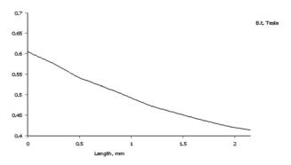
Fig. 18: Tangential flux density diagram in winding area, through the magnet axis
