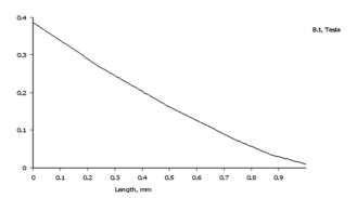
Fig. 33: Tangential flux density diagram in the stator core area, through the magnet axis
