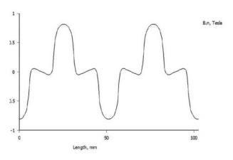
Fig. 4: Flux density diagram in the air-gap, in the proximity of the permanent magnet
