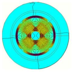
Fig. 22: Torque motor with a large air-gap in load conditions at 1A – magnetic field distribution
