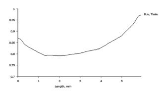
Fig. 41: Normal flux density diagram, transversal on the magnet, in the middle area
