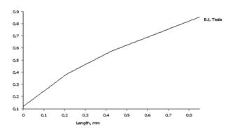
Fig. 10: Tangential flux density diagram in the rotor hub, through the magnet axis  $\,$
