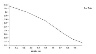
Fig. 48: Normal flux density diagram in the stator core area, through the magnet axis
