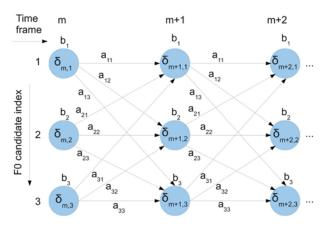
Fig. 1: The trellis of the Viterbi algorithm
