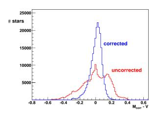
Fig. 5: Distribution of the difference between the measured reference star magnitudo and the catalogue V magnitudo before (red) and after (blue) spectral correction
