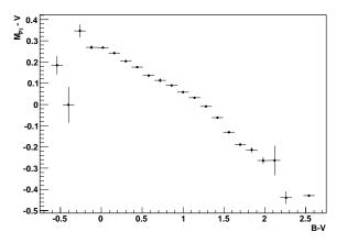
Fig. 4: Average difference between the "Pi of the Sky" magnitudo  $M_{Pi}$  and the catalogue V magnitudo for the reference stars, as a function of the spectral type given by B - V
