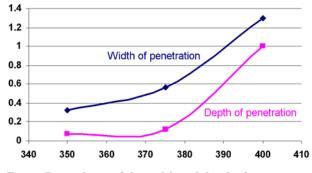
Fig. 8: Dependence of the width and depth of penetration on the excitation voltage
