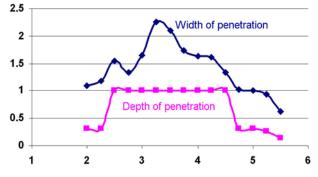
Fig. 9: Influence of the focal length on the geometry of the penetration passes
