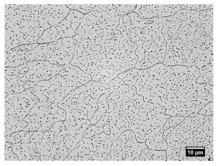
Fig. 6: Microstructure weld metal (Al 99.50 %)
