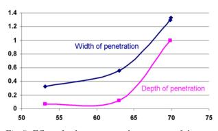
Fig. 7: Effect of pulse energy on the geometry of the penetration passes
