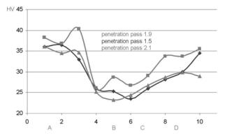
Fig. 10: Graphic illustration of the course of microhardness on samples 1.5, 1.9, 2.1 A – parent material, B – heat-affected zone, C – boundary of smelting, D – weld metal
