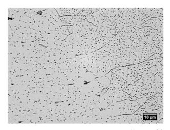
Fig. 5: Microstructure the heat-affected zone (Al 99.50 %)
