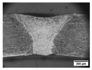
Fig. 4: Penetration pass 1.5
