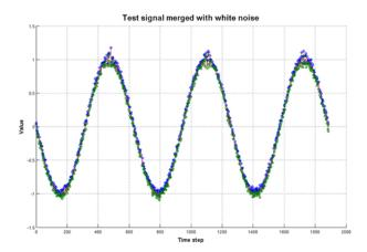
Fig. 5: Test signal with white noise added (red dashed line) and the location of its highs (blue circle) and lows (green circle)
