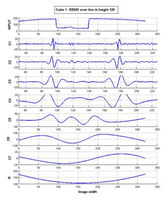
Fig. 10: Cube 1 – All IMF functions extracted by EEMD
