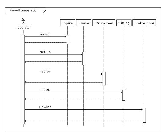
Fig. 4: Sequence diagram describing preparation for unwinding
