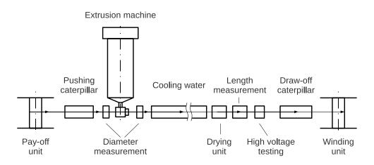
Fig. 1: NFA2X cable core processing line
