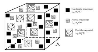
Fig. 2: A scheme of a porous composite material (3 components)
