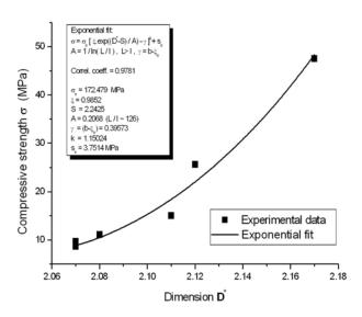
Fig. 1: Dependence of compressive strength on fractal dimension with cement paste [8]
