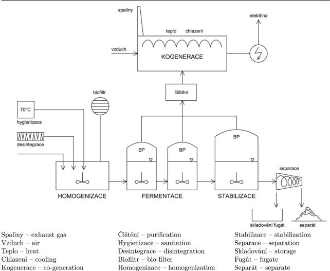
Fig. 1: Simplified scheme of a biogas plant
