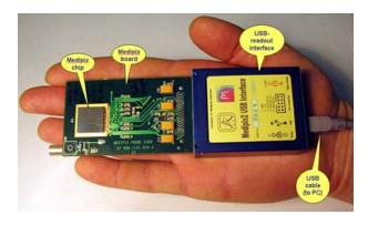
Fig. 1: Medipix2/USB-interface radiation camera. The Medipix board (left) is attached to the USB-based readout interface (right)
