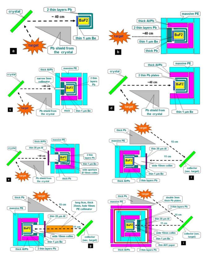
Fig. 8: Schematic illustration of the target and shield setups investigated for the  $BaF_2$  detector. The geometric setup is determined by the position of the primary target, the (eventual) crystal/collector as a secondary target, and the detector. The shield assembly was composed of materials with polyethylene (PE), lead (Pb), Aluminum (Al), a thin Beryllium (Be) foil window in various segment sizes and thicknesses
