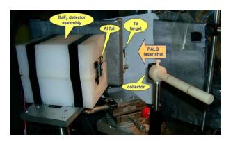
Fig. 7: Indirect experimental setup in the PALS interaction chamber: The  ${\rm BaF_2}$  detector assembly, facing the secondary target – the collector, is shielded from the primary Ta target
