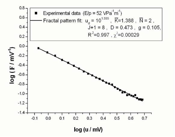
Fig. 4: Fractal pattern fit of population statistics (voltage pulses – data taken from Fig. 2). The quantity  $\overline{u}_d = 10^{1.555}$  mV is a voltage scale corresponding to the average voltage pulse created by the largest avalanches detected. The quantity g is not a normalization constant but only indicates the shift between unnormalized data and the unnormalized distribution F(n,d). After [14].
