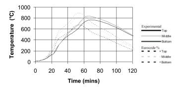
Fig. 1: EC % method: flexible end plate
