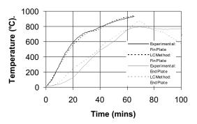
Fig. 3: Lumped capacitance method for fin plate and flexible end plate
