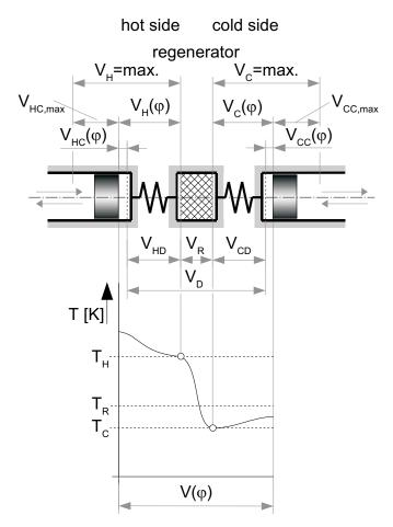
Fig. 1: Scheme of a Stirling engine with dead volumes and progress of the temperature of the working gas for crank angle  $\varphi$
