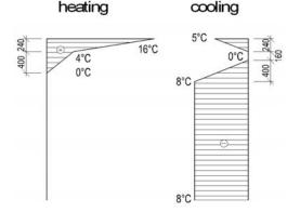
Fig. 7: Temperature gradient in the vertical direction, according to ENV 1991-2-5
