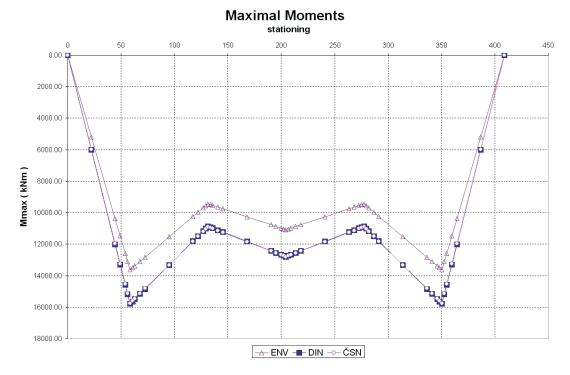
Fig. 10: Maximum moments from temperature loading
