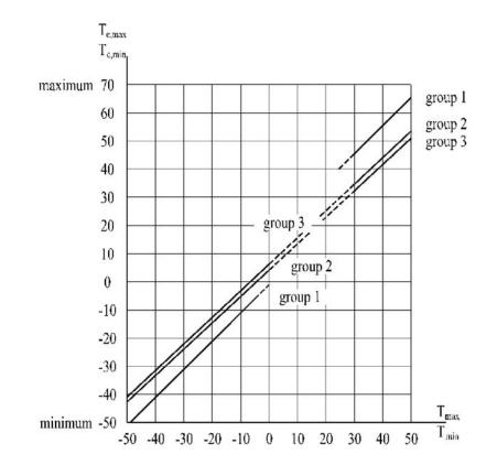
Fig. 2: Correlation between shade air temperature and structure temperature
