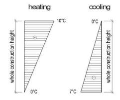
Fig. 8: Temperature gradient in the vertical direction, according to DIN 1072
