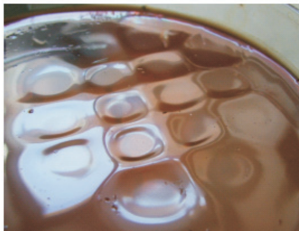
Fig. 3: Photograph of a Petri dish showing the gel surface deformation caused by the corona discharge exposition
