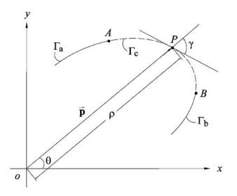
Fig. 1: Blending of two curve segments with a third one
