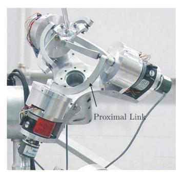
Fig. 2: Prototype of the Agile Wrist
