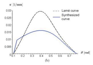
Fig. 8: (a) New housing profile and (b) curvature distribution over the synthesized curve; shown dashed is the Lamé curve
