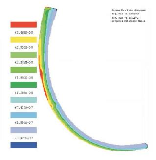
Fig. 5: Von Mises stress distribution along the optimized proximal link (thickest cross-section is located closest to the motor)
