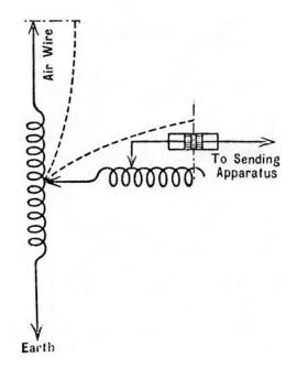
Fig. 6: Connections at receiving station
