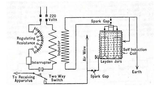
Fig. 5: Connections at transmitting station
