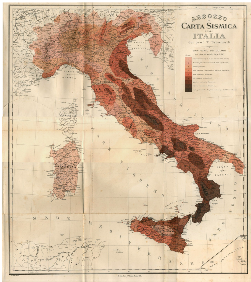
Figure 3. The 'Abbozzo di Carta Sismica della Italia' ('Draft of a Seismic Map of Italy'), compiled in 1886 by early Italian geologist Torquato Taramelli (1845-1922), subdivided the Italian seismogenic areas based on the number of earthquake occurrences per century, starting with the year 1300. It is perhaps the oldest ancestor of the current probabilistic seismic hazard maps [Taramelli, 1886].
