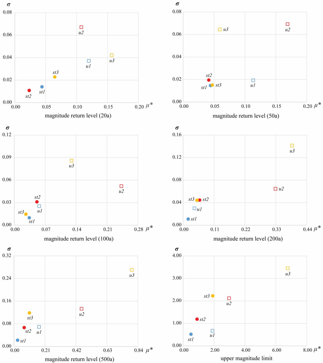
Figure 7. Absolute means ( \mu^* ) and standard deviations ( \sigma ) of the elementary effects of the two input factors for magnitude return levels, upper magnitude limit and their corresponding confidence intervals ( u1 and st1 represent the input factors for magnitude return levels or upper magnitude limit. u2 and st2 represent the input factors for low end of confidence interval. u3 and st3 represent the input factors for upper end of confidence interval).
