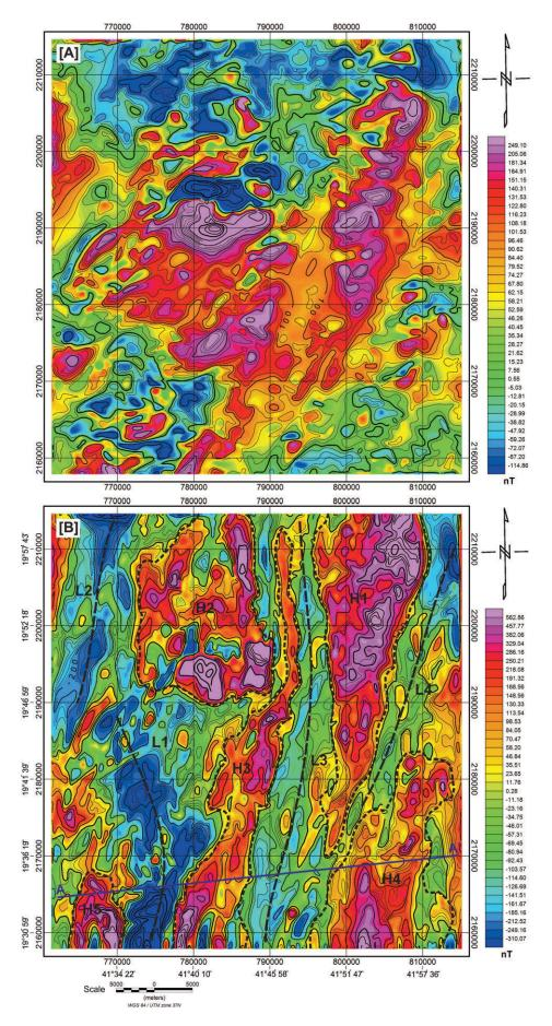
FIGURE 3. Interpretation of reduce to pole anomaly zone map. [A] Total Magnetic Intensity (TMI) map of the Biljurshi study area. [B] Interpreted reduce to pole (RTP) map with location of the studied sections AA.
