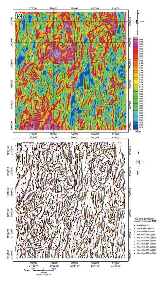
FIGURE 4. [A] Horizontal Gradient Magnitude (HGM) map of the Biljurshi study area and extracted lineaments. [B] Maxima of horizontal gradient magnitude (HGM) combined with the extracted lineaments, showing dip of the geologic contacts.
