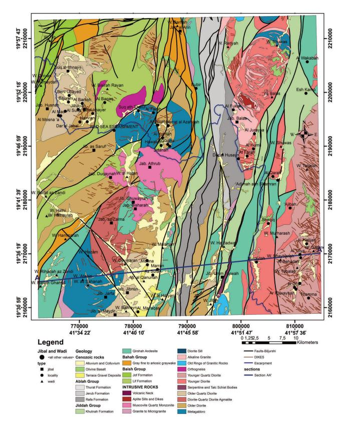
FIGURE 2. Extract of the Biljurshi geological map (1:100 000, resized), showing relation between the Umm Farwah master fault and the associated volcanic, sedimentary and metamorphic rocks and intrusive bodies.
