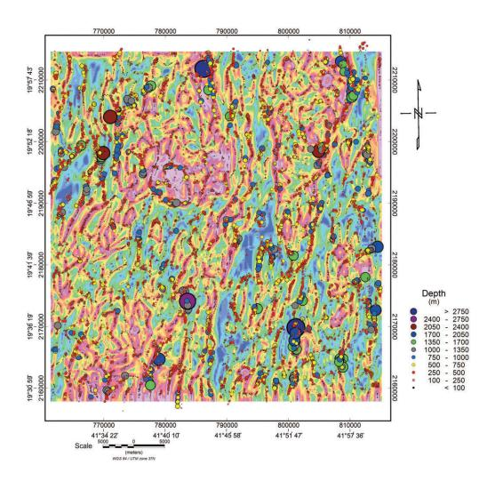
FIGURE 5. Euler solutions (SI =0) of RTP magnetic anomaly zone, showing estimated depth for highlighted geological contacts.
