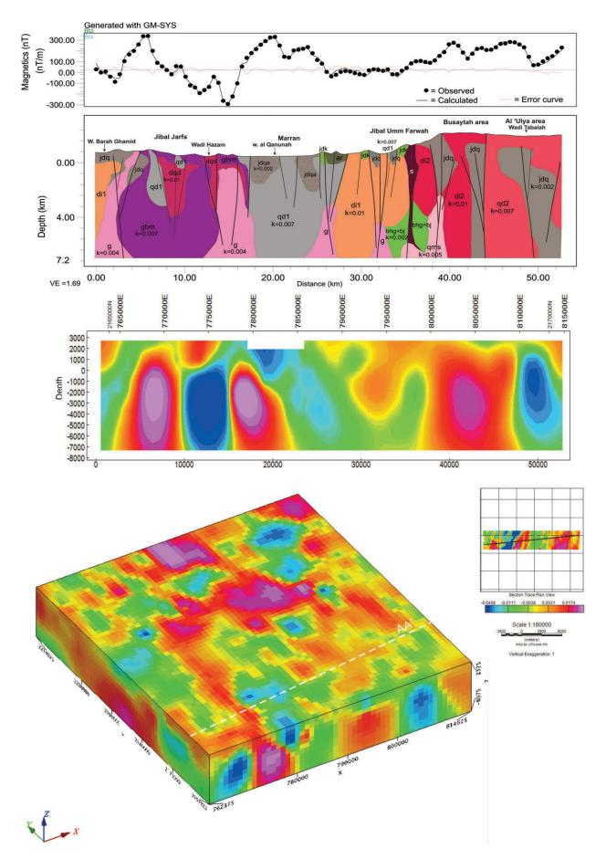
FIGURE 7. Inversion model of the study area, obtained from RTP magnetic data, showing the susceptibility contrast in depth. The inversion section AA', extracted from 3D inversion model obtained by 3D VOXI, is superimposed by the 2D forward model.
