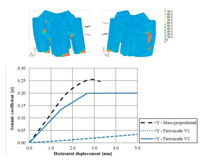
**FIGURE 19.** Comparison of capacity curves obtained with pushover proportional to first–mode "V1" and "V2" (blue color), with respect to the mass–proportional pushover capacity curve (black color) in the +*Y* direction.
