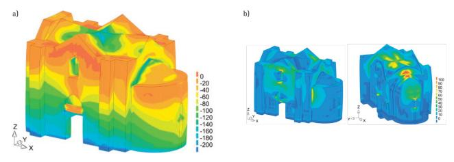
**FIGURE 15.** Deformed shape and distribution of (a) minimum (compressive) and (b) maximum (tensile) principal stresses, due to self–weight (in the last picture, the stresses are plotted on the internal surfaces of the vault and of north and east walls). Units: kPa.
