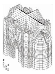
FIGURE 12. Views of the finite element mesh of the Church.
