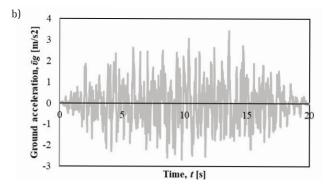
FIGURE 21. Unscaled time-history of accelerations with a PGA of 3.4 m/s<sup>2</sup>, applied in the (a) X and (b) Y directions.
