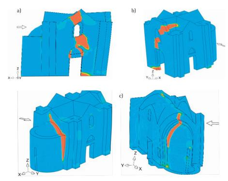
**FIGURE 18.** Deformed shape and cracking, given the maximum principal strain  $\varepsilon_1$ , based on pushover analysis. The results correspond to the following loading patterns: (a) "(+X)+(0.3 Y)", (b) "(-X)+(0.3 Y)", and (c) "+Y". The direction of the full mass–proportional load is given by the orientation of the white arrows, while the shaded arrows show the direction of the combined 30% loading.
