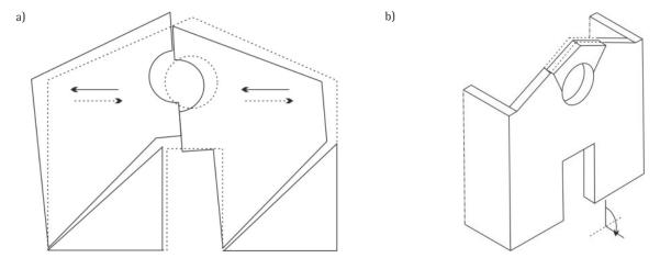
**FIGURE 23.** Typical seismic failure mechanisms of churches according to the Damage Abacus [NIKER, 2010]. In–plane shear fail—ure mechanism of (a) the whole façade or (b) of the top section of the window.
