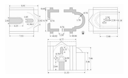
FIGURE 3. Geometry of the Armenian Church. Units: m.
