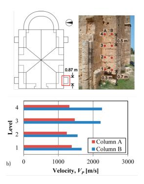
FIGURE 11. Direct testing locations, grids and measured velocities of the (a) south wall and (b) southwest buttress.
