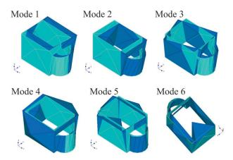
**FIGURE 10.** Experimental mode shape identified by means of the software ARTeMIS Modal Pro.
