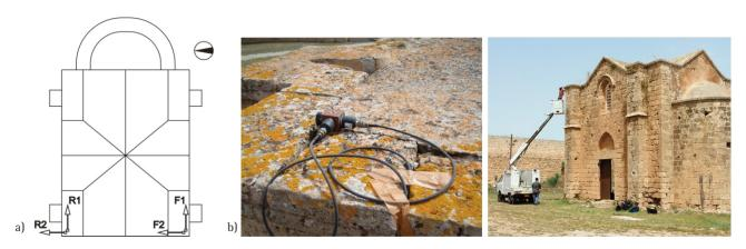
**FIGURE 9.** Dynamic identification. (a) One of the test setups showing the position of the reference (*R*) and free (*F*) accelerometers; and (b) views of the dynamic measurements.
