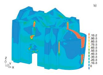
**FIGURE 16.** Capacity of the building against vertical loading. (a) force–vertical displacement diagram, plotted at the top of the apse (units: m); and (b) deformed shape and cracking, given by the maximum principal strain  $\epsilon_1$ , due to vertical loading, at maximum capacity.
