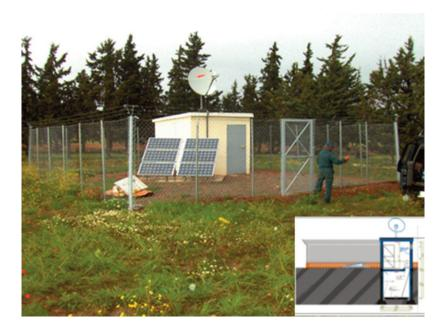
**Figure 4.** Example of a VSAT two-levels seismic vault, showing the VSAT data-transmission parabola and solar panels. The schematic diagram on the bottom-right shows an overall sketch of a station with the lower level at a depth below surface-level.
