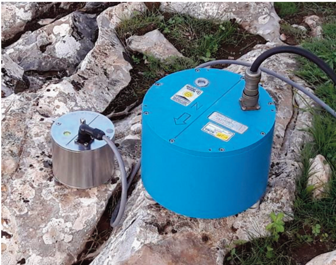
Figure 8. The ETL3D/5s sensor (left) and the reference Lennartz LE-3D 5/S (right) during the test.
