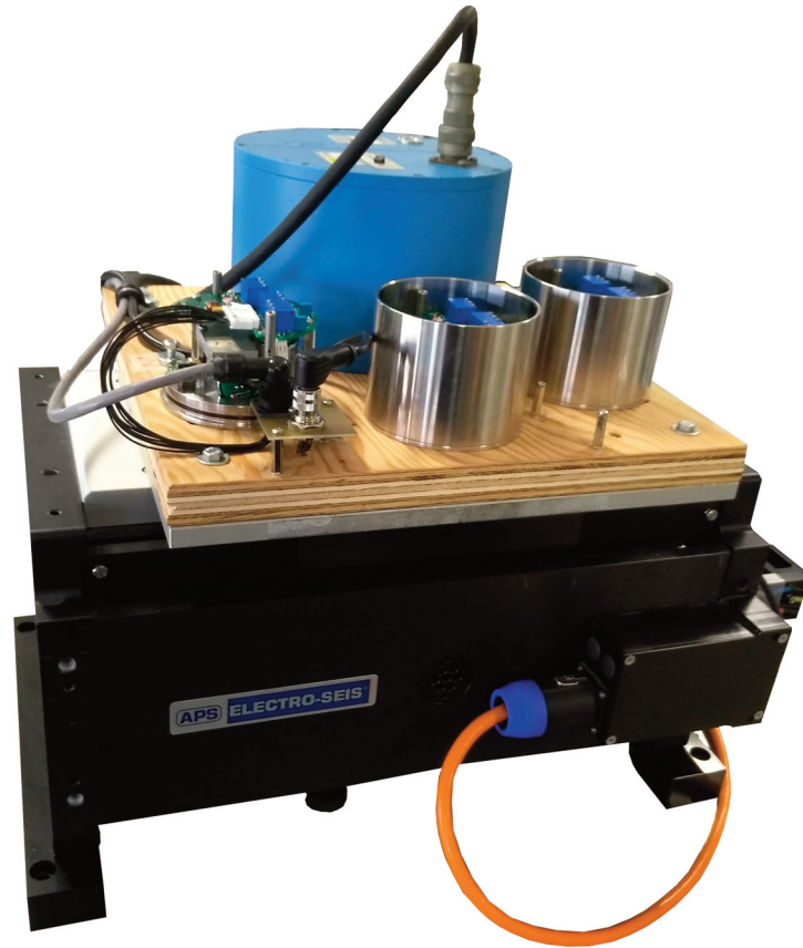
Figure 5. A set of three ETL3D/5 sensors mounted on a shaking table, along with a Lennartz LE 3D 5s (blue case). The latter acts as a reference velocity sensor. The shaking table has been provided by Kore, the University of Enna.
