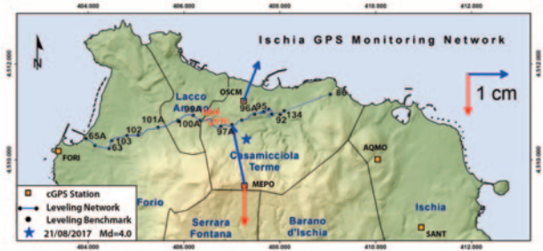
FIGURE 15. Sketch of the cGPS network of Ischia Island on which the “Borbonica Line” is overlapped. The vertical and horizontal coseismic displacements are indicated by the red and blue arrows respectively, recorded at the OSCM and MEPO stations following the earthquake of 21 August 2017 (Md = 4.0) [INGV/Osservatorio Vesuviano, Settembre 2017, modified].
