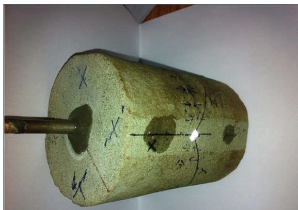
FIGURE 17. Fracture orientation as seen on sample surface.
