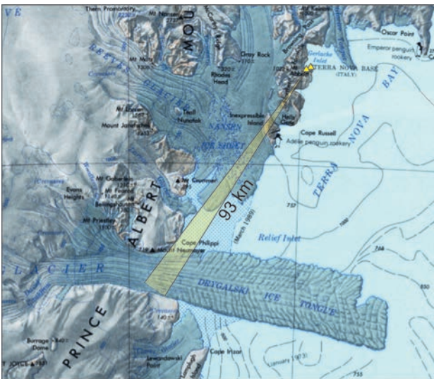
Figure 10. Approximated source location by using the source azimuth (black line and yellow area) and the source-station distance, calculated by the S-P differential times. Yellow triangles represent the two seismic stations STN01 and STN02.
