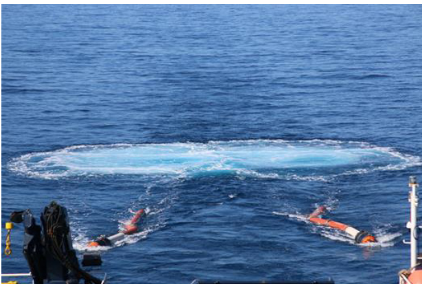
Figure 10. A picture of the real bubble generated by the air-guns mounted in the vessel “Sarmiento de Gamboa”.
