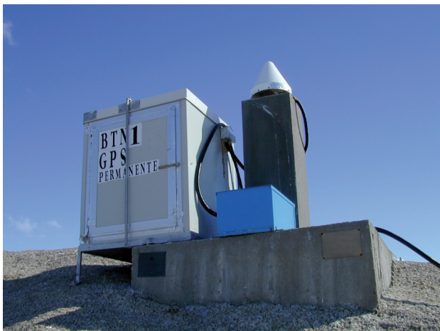
Figure 1. The TNB1 permanent GPS station, the antenna and its cone radome, and the shelter that contains the Ashetch-ZXII receiver and the ancillary equipment.
