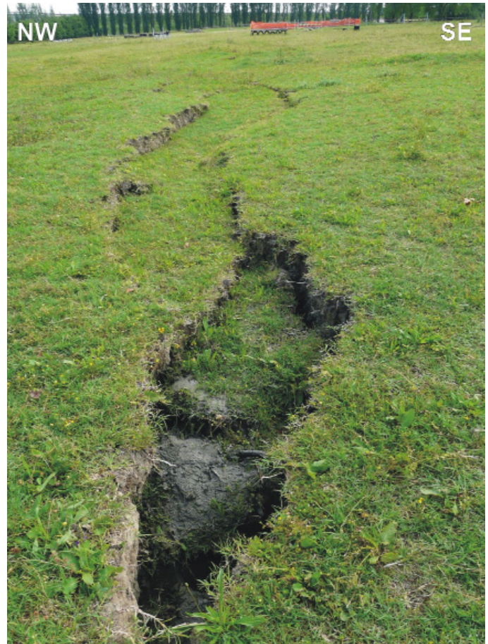
Figure 2. Example of a small-scale graben formed along the fracture system that developed on the levee of the paleo-reach of the Reno River, close to the trench site. See Figure 1 for location.
