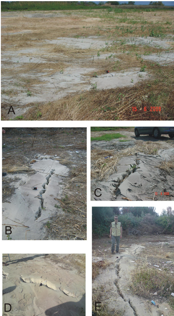
Figure 7 (left, top to bottom). Liquefaction manifestations at the sea shore of the village Kato Achaia. (a) General view of the area; (b,c,d) examples of vent fractures with 12, 20 and 30 cm-width, respectively; (e) formation of a 4 m-long vent fracture.
