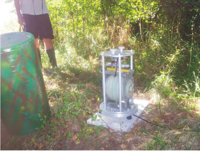
Figure 1. The DIDD device on levelled marble plate in Krbavsko Polje station. The green cylinder on the left is the instrument case which protects the instrument against humidity and improves the temperature stability.
