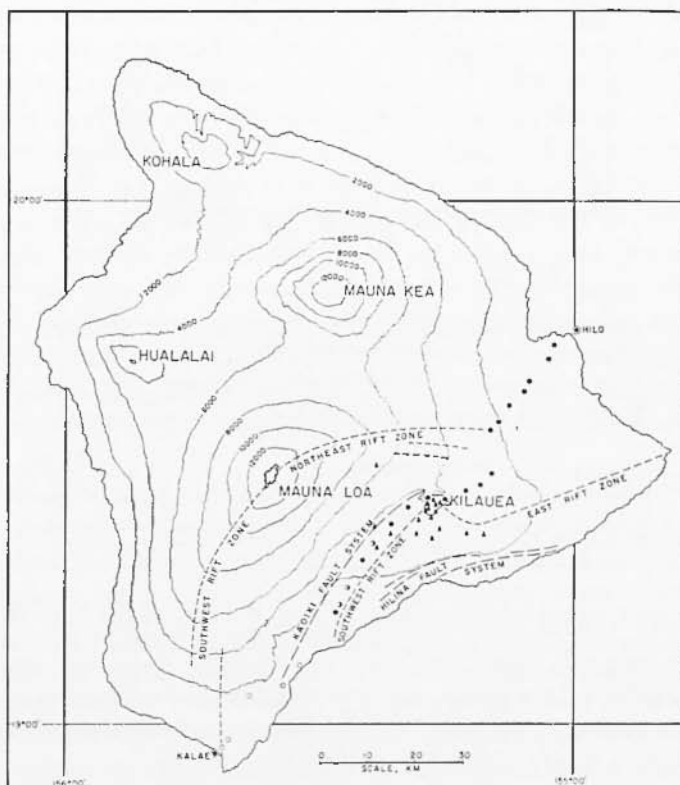
Fig. 3. — A topographic map of the island of Hawaii in the Hawaiian Islands. Elevations are in feet. Rift zones are denoted by short-dashed lines; fault systems, by long-dashed lines. Circled dots show location of the shotpoints; solid triangles show locations of the fixed stations. Solid dots are temporary stations for the Hilo shots; open circles are temporary stations for the Kalae shots. Circles that are half-closed show locations of temporary stations used for both shot series [from Ryall and Bennet ( 27 )].
