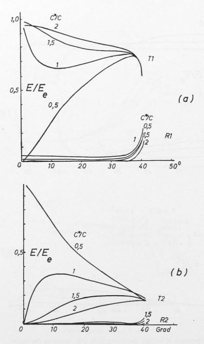
Fig. 10 - Energy ratios. Influence of varying the ratio  $C^*/C$ . For the other constants see Fig. 9.
