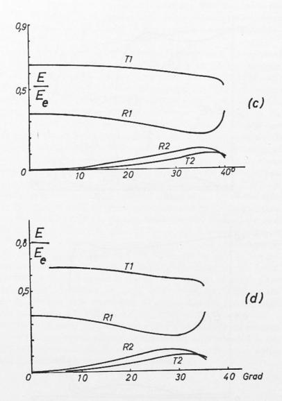
Fig. 3 - The energy ratios for ice/schists.
