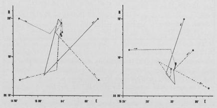
Fig. 2 - The figure shows the independence of the calculated epicenter from the preliminary position attributed to it.
