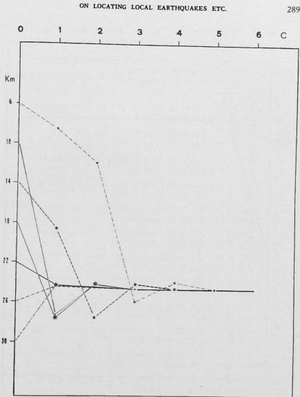
Fig. 3 a, b - The depth values obtained in the calculation for each iteration and the good convergence of h to a definitive value.
