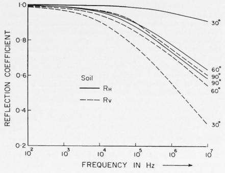
Fig. 1a, b, c, d, e) - Frequency variation of  $R_v$  and  $R_h$  for soil, shale, dolomite, gabbro and quartzite.
