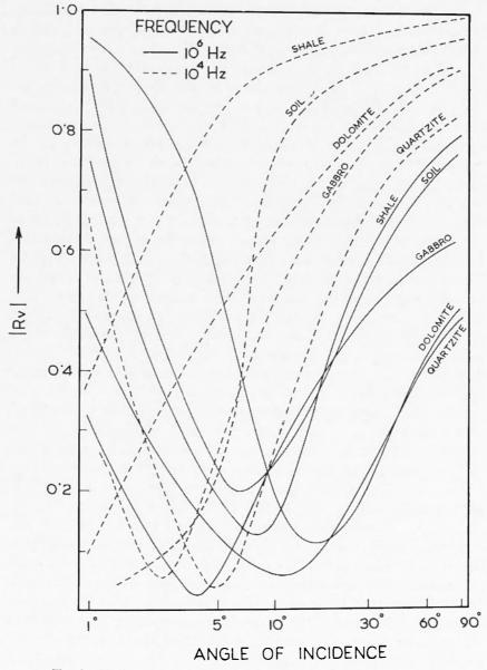
Fig. 2 - Variation of  $R_{\rm e}$  with angle of incidence for soil, shale dolomite, gabbro and quartizite.
