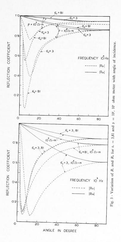
cross over and reversal in the magnitude takes place, but the values are closed to each other. The characteristic features of  $R_h$ and  $R_v$ , variations discussed above are retained at 10<sup>5</sup> Hz but the variation in magnitude is large for  $R_h$ , whereas for  $R_v$ , the mininum magnitude is more or less or equal for all cases.
