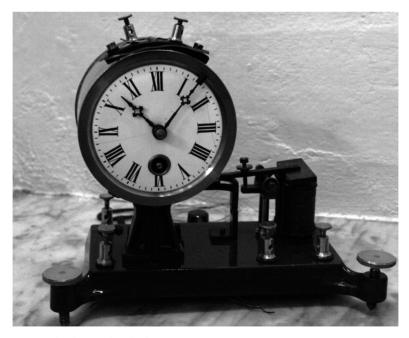
Fig. 2. Galli-Brassart seismic worning device.
