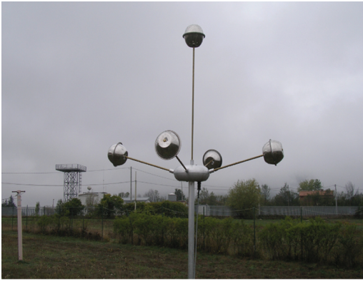
Fig. 3. Three-axes electrometer for the measurement of the atmospheric electric field in the frequency band [1 Hz-100 kHz]. The instrumental sensitivity is 1 \mu\text{V}/(\text{m}\sqrt{\text{Hz}}) .
