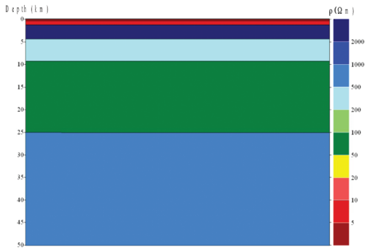
Fig. 4. 1D resistivity model structure of the subsurface in the area of L’Aquila Observatory.
