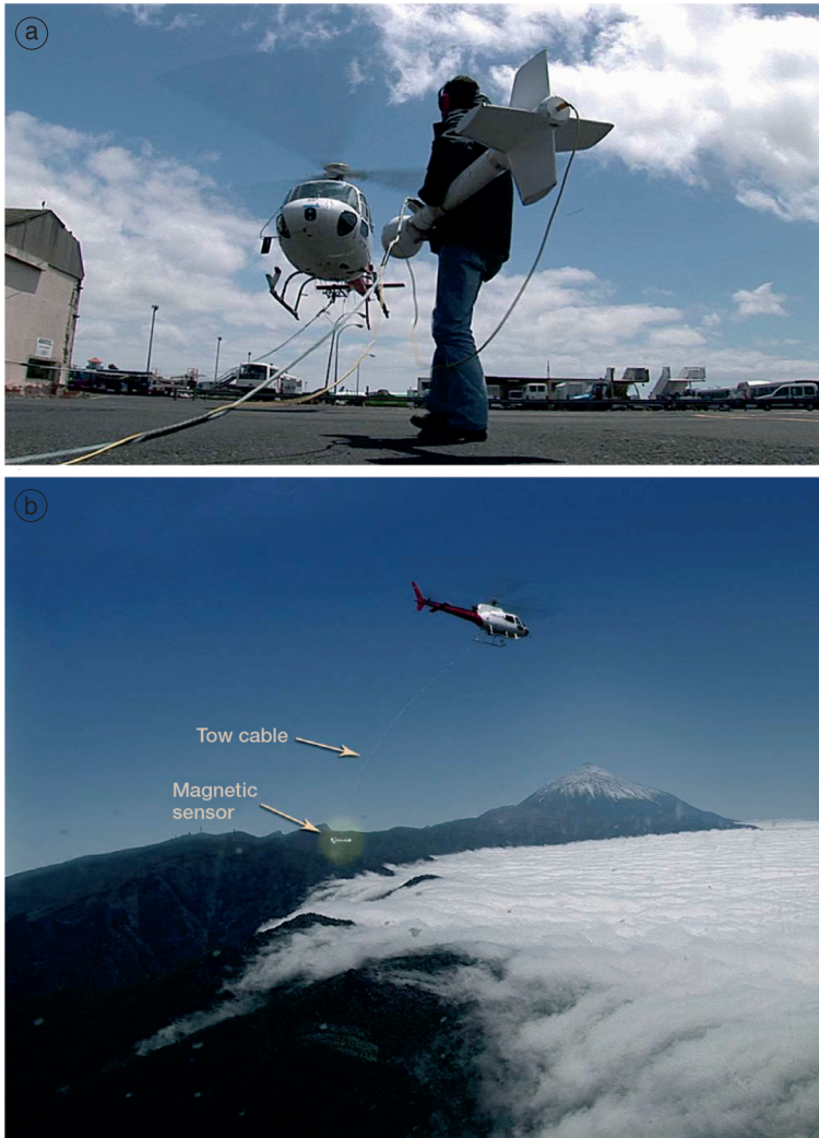
Fig. 2a,b. a) Logistical operations during takoff and landing for launching and retrieving the towed airborne magnetometer bird attached to the barycentre hook of the Aerospatiale Squirrel AS 350 helicopter; b) magnetic sensor and tow cable while airborne with the Teide volcano in the background.
