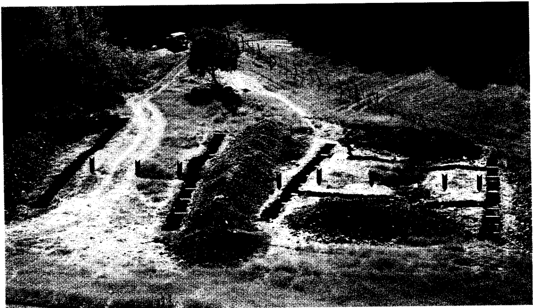
Fig. 8. Trench site on the Rodgers Creek strike slip fault (North San Francisco bay). The fault runs across this little alluvial basin (the main fault trace is indicated by arrows) and forms a little pressure ridge clearly cut by the two trenches on the left. Two sets of trenches have been opened, parallel and perpendicular to the fault, to investigate the slip along the fault by reconstructing piercing lines and recognize the occurrence of repeated faulting events as recorded in the fault zone. Trenches are about 1 m-wide and are shored by using hydraulic jacks set each 2 m.
