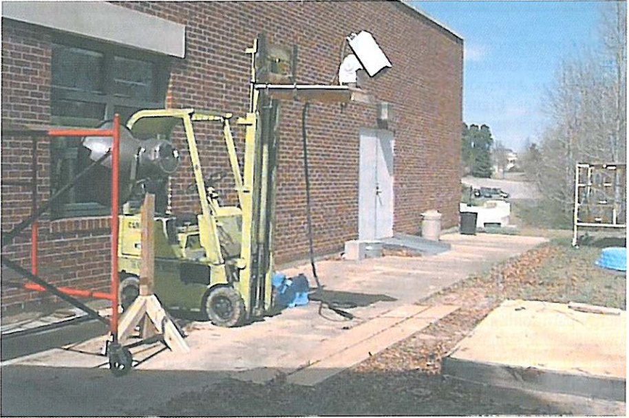
Fig. 5. System set-up for outdoor measurements of acoustic to seismic coupling over objects buried in sand.
